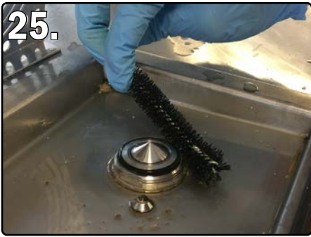
25. SCRUB AROUND EXPOSED VALVES AND RINSE CLEAN
