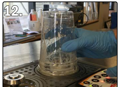
12. THE LINE WILL "POP" AND CLEANER WILL START FLOWING THROUGH THE LINE
