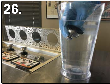
26. RINSE OFF NOZZLES IN BOTH UP & DOWN POSITION (SINK OR PITCHER WILL WORK)
